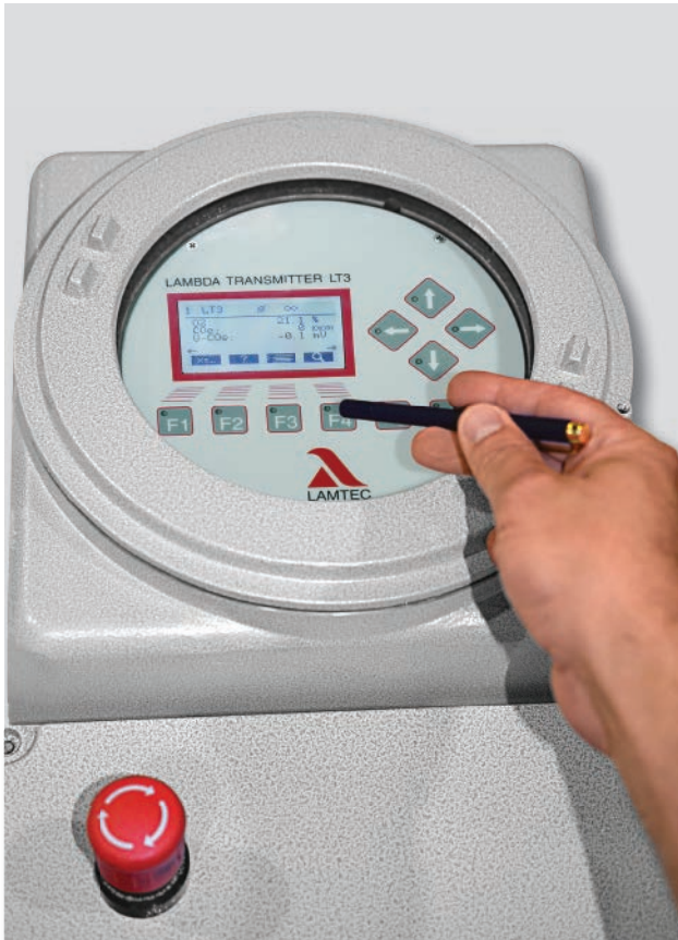
Operation using magnetic pin.
