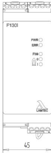
Fig. 1-2 dimensions F130I Housing material: Plastic
