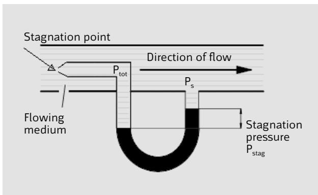
$P_{\text{tot}}$  = overall pressure,  $P_s$  = static pressure,  $P_{\text{dyn}}$  = dynamic pressure (stagnation pressure).
