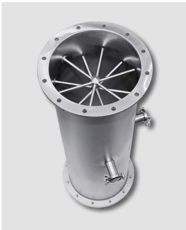
The principle of the mass flow measurement grid follows the Bernoulli energy equation on which the principle of the conservation of energy is based. The entire kinetic flow energy (without friction losses) remains constant as the sum of the dynamic and static pressure. As a differential pressure flow metering method, the mass flow measurement grid records the overall pressure and static pressure of a flowing gas.
