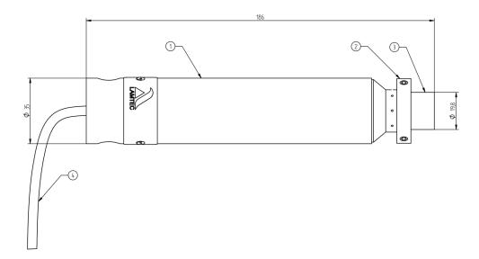
Fig. 2 Lambda Probe LS2 ECO (dimensions in mm)
