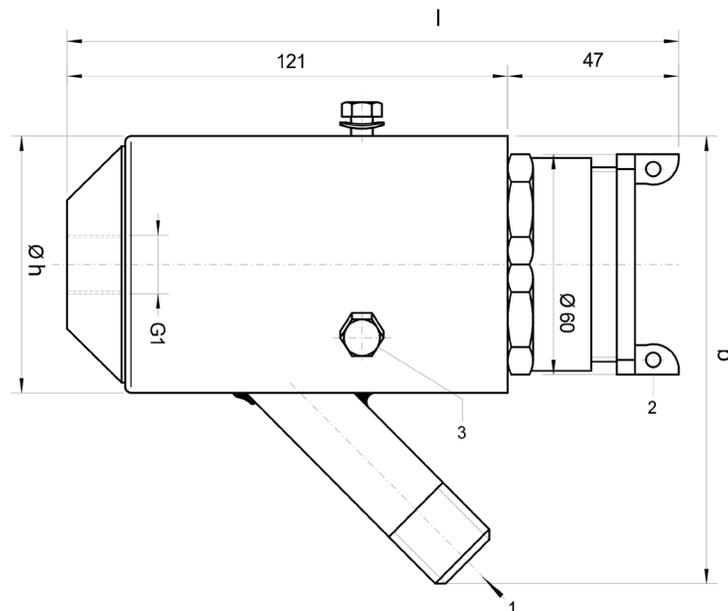
Dimensional drawing cooling air Housing FS30
