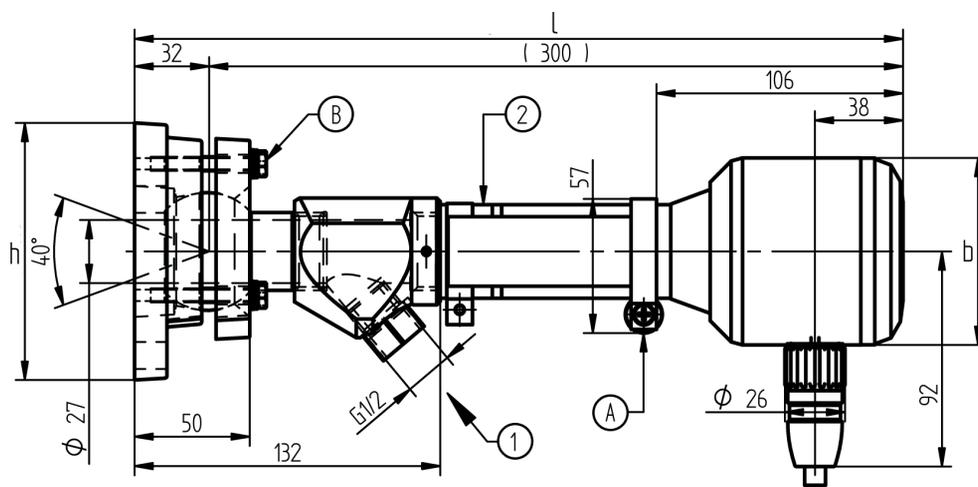
Dimensional drawing FH40-10 with flame scanner F200K
