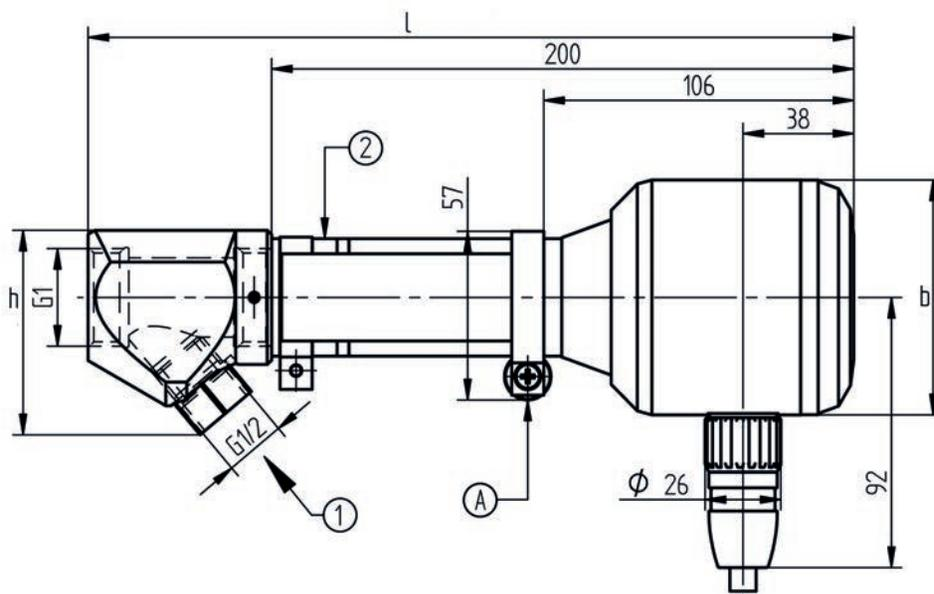
Dimensional drawing FH30-10 with flame scanner F200K
