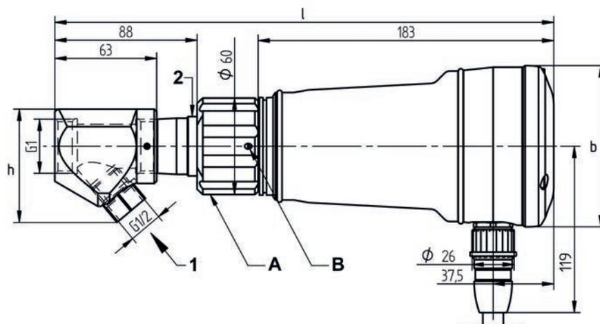
Dimensional drawing FV30-10 with flame scanner F300K
