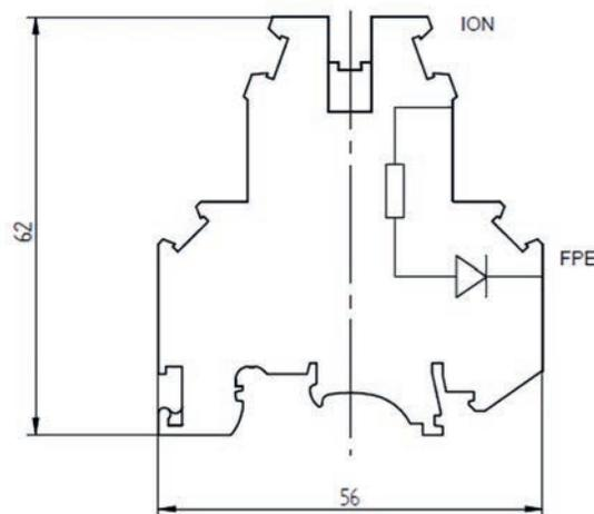
Dimensional drawing 2-level terminal ionisation block
