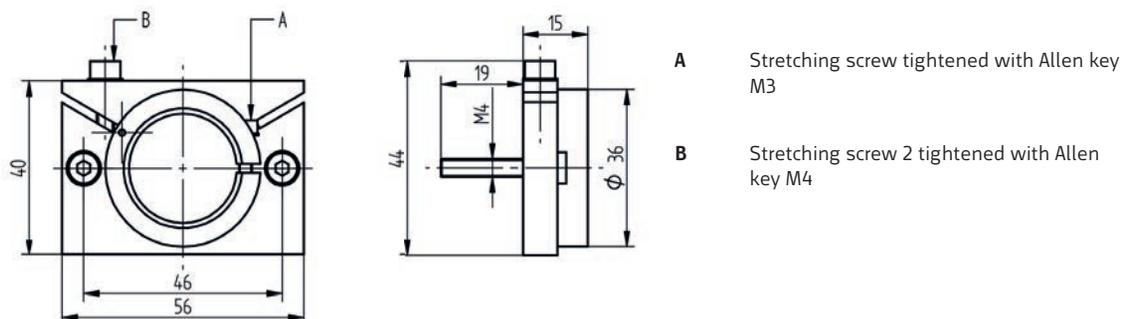
Dimensional drawing Adjustment bracket for direct attachment to the burner
