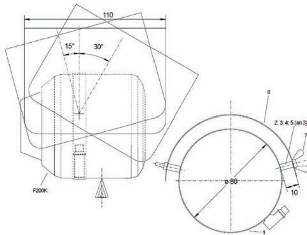
Dimensional drawing weather protection FW 01 for F200K
