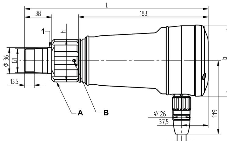
Dimensional drawing FV30-00 with flame scanner F300K
