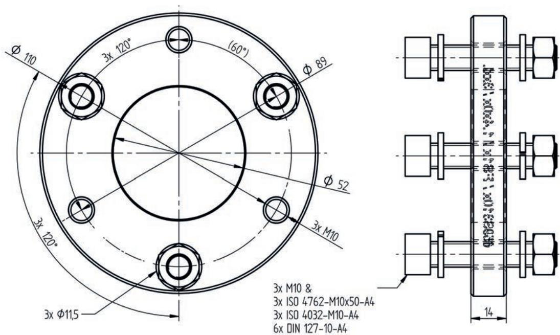
Dimensional drawing Welding neck flange FS1x in V4A and V2A
