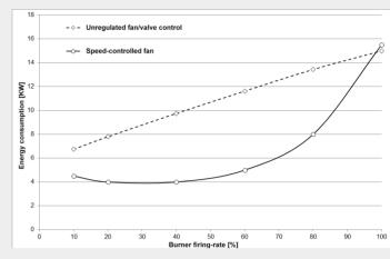
Fig. 7: Comparison of the energy consumption of the unregulated and speed-controlled combustion air fan via the burner load
