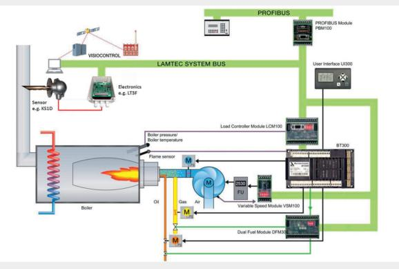
**Fig. 5**: Boiler with dual-fuel burner equipped with BurnerTronic BT300, speed control, in-situ gas sensor and sensor electronics for optimise CO<sub>a</sub>/O<sub>2</sub>
