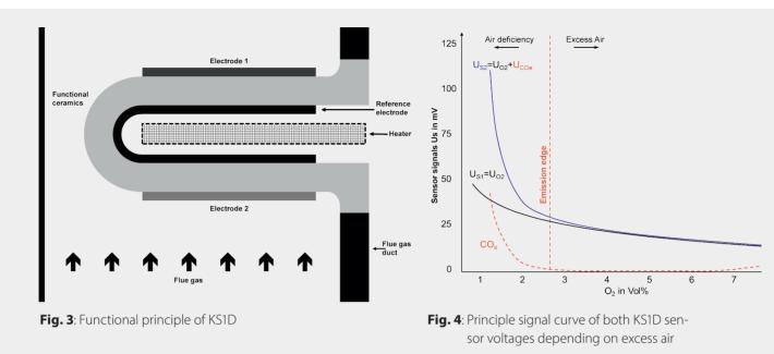
A typical CO<sub>e</sub> curve when slowly reducing O<sub>2</sub> and hence heading towards incomplete/bad combustion shows a significant increase of combustibles  $CO_e$  at the emission edge due to a lack of combustion air (also refer to Fig. 1).
