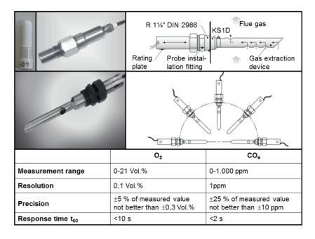
Fig. 2: Combination probe KS1D for the simultaneous measurement of  $\rm O_2$  and  $\rm CO_e$
