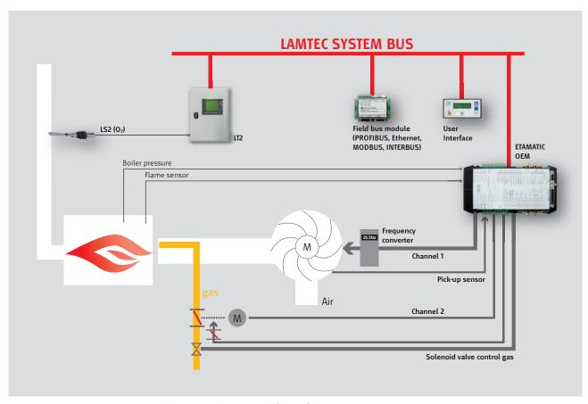
Functions in the LAMTEC ETAMATIC OEM burner control with O<sub>2</sub> trim (LT2/LS2).
