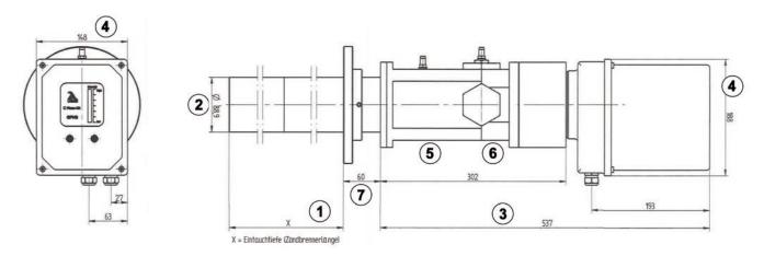
Fig. 2 Dimensions of GFI70 pilot burner design A/B
