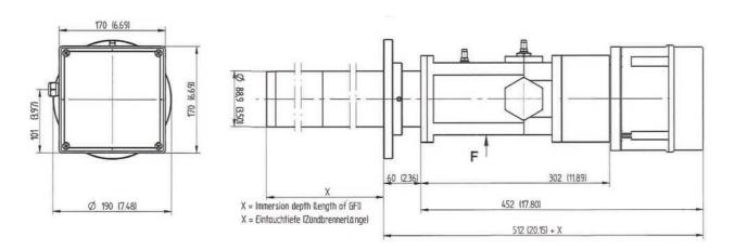
Fig. 4 Dimensions of GFI70 pilot burner Ex-Zone 2
