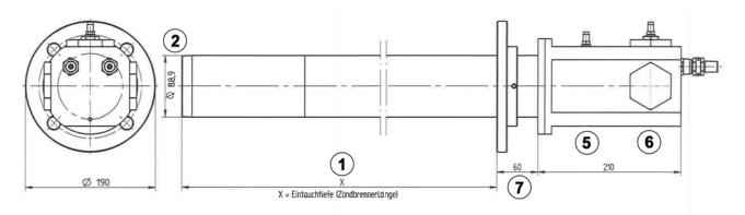
Fig. 6 Dimensions of GFI89 pilot burner design C
