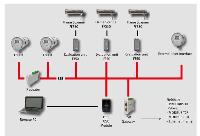
Example: Connection of multiple flame scanner systems. F350 can be combined with the F300K without a problem.
