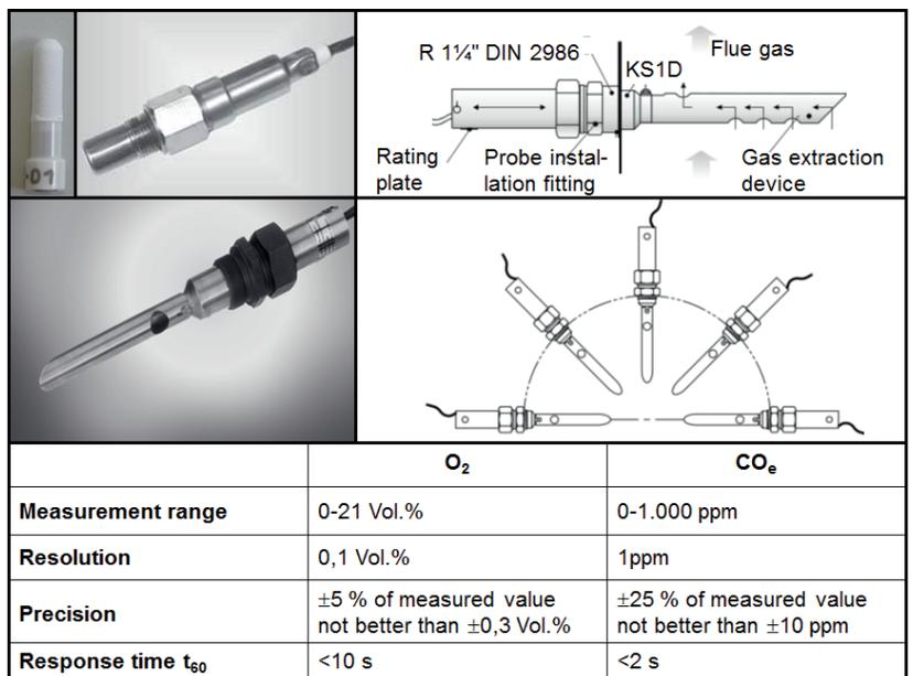
Fig. 2: Combination probe KS1D for the simultaneous measurement of O<sub>2</sub> and CO<sub>e</sub>
