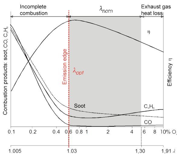
**Fig. 1:** Typical curve of the pollutant emissions and efficiency depending on excess air
