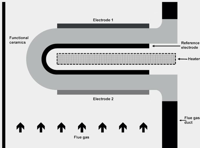
Fig. 3: Functional principle of KS1D
