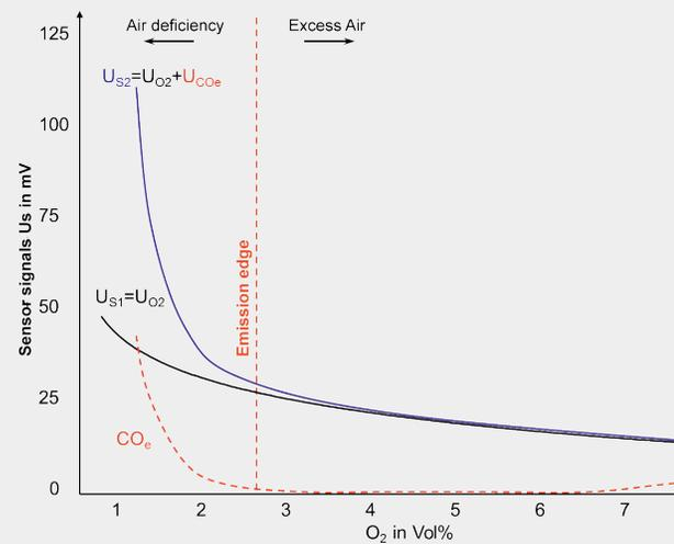
Fig. 4: Principle signal curve of both KS1D sensor voltages depending on excess air
