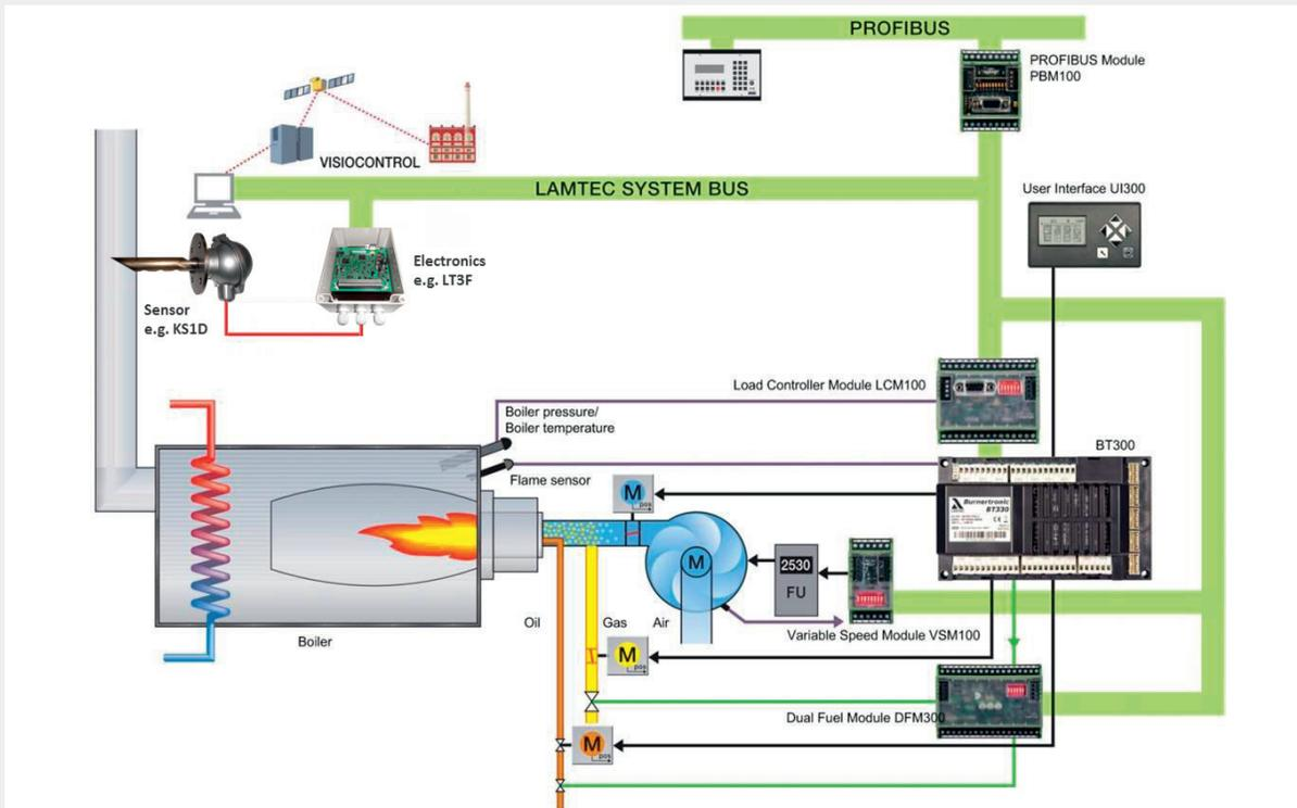
**Fig. 5:** Boiler with dual-fuel burner equipped with BurnerTronic BT300, speed control, in-situ gas sensor and sensor electronics for optimise CO<sub>e</sub>/O<sub>2</sub>
