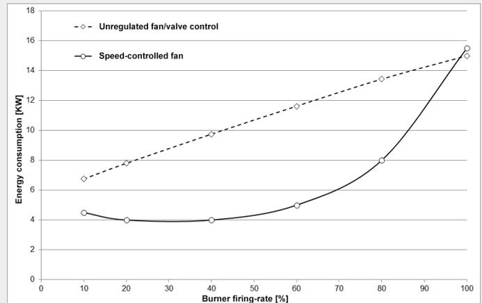
**Fig. 7:** Comparison of the energy consumption of the unregulated and speed-controlled combustion air fan via the burner load
