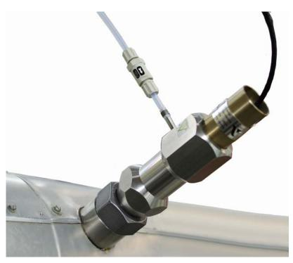
Fig. 7 Testing device plugged into flue gas channel
