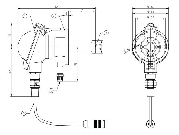
Fig. 2 Combination Probe KS1D-HT (dimensions in mm)
