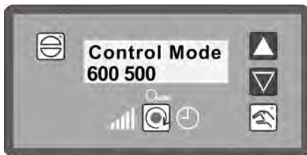
Fig. 5-2 Display with external burner-firing-rate-controller
