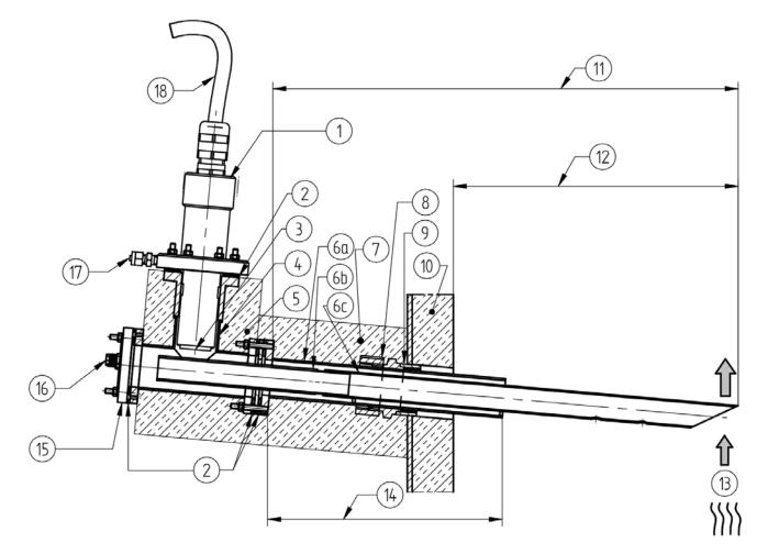
Fig. 4 Ex Probe with GED FLEX made of Inconel or stainless steel with T-adapter
