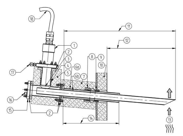
Fig. 5 Ex Probe with GED FLEX made of Kanthal or AL203 with T-adapter
