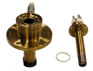
Fig. 7-6 Dismounted sensor with seal
