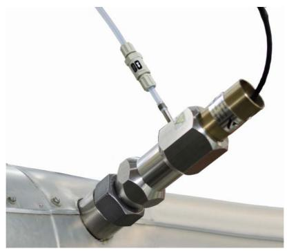
Fig. 7-2 Testing device plugged into flue gas channel
