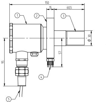
Fig. 2 Dimensional drawing Lambda Probe LS2-BF
