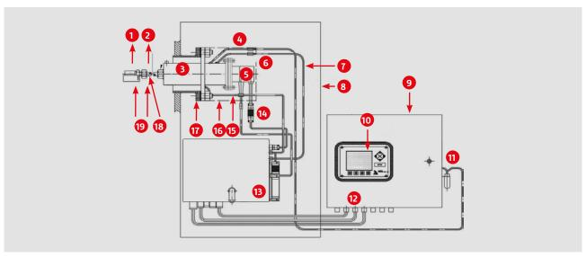
Design principle with external measuring gas pump and calibration system.
