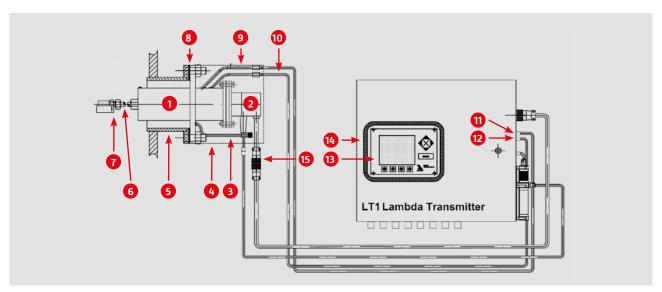
Design principle with integrated measuring gas pump and calibration system for installation under cover.
