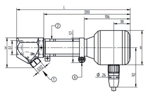
Dimensional drawing FH30-10 with flame scanner F200K
