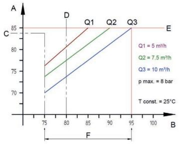
Performance characteristics cooling air housing FK30 at cooling air temperature 25 °C
