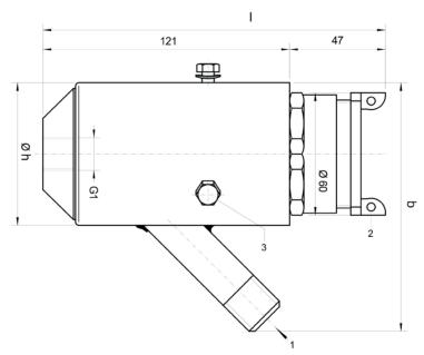
Dimensional drawing cooling air Housing FS30
