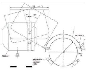
Dimensional drawing weather protection FW 01 for F200K
