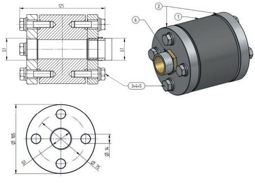
Dimensional drawing Vibration Decoupler
