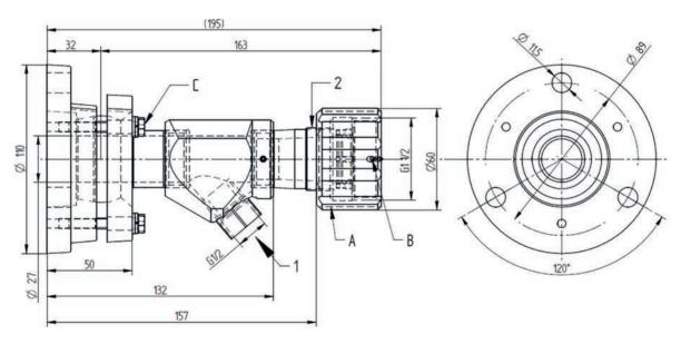
Dimensional drawing FV40-15 excess Pressure
