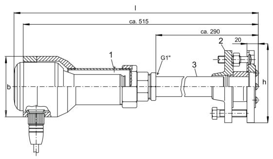
Dimensional drawing FS56 with flame scanner F200K
