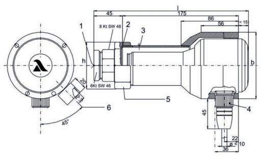
Dimensional drawing FS50 with flame scanner F200K
