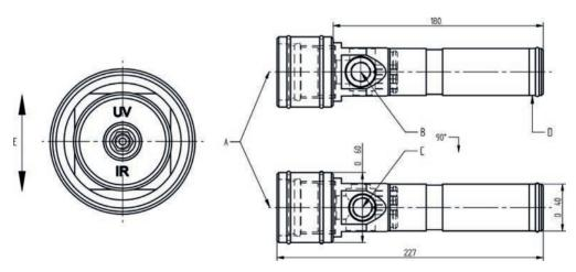
Dimensional drawing Flame Scanner Testing Device FFP30
