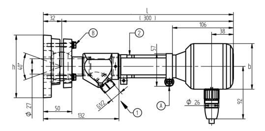
Dimensional drawing FH40-10 with flame scanner F200K
