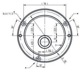
Dimensional drawing External User Interface FB 30-10 - mounting on the control cabinet door
