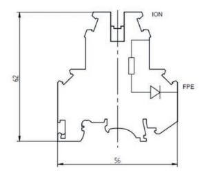
Dimensional drawing 2-level terminal ionisation block
