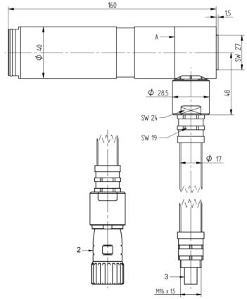
$Dimensional\ Drawing\ FFS07\ with\ metal\ protection\ hose,\ FFS07\ for\ screw\ fitting,\ not\ available\ for\ FFS07...\ Experimentary and the protection of the protection$
