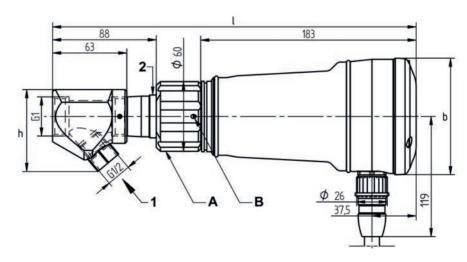
Dimensional drawing FV30-10 with flame scanner F300K
