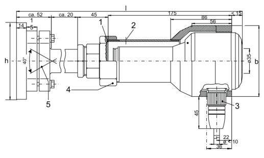
Dimensional drawing FS51 with flame scanner F200K
