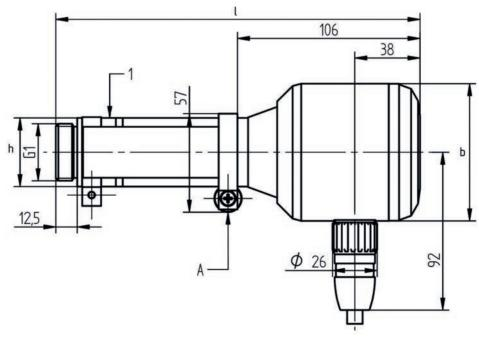
Dimensional drawing FH30-00 with flame scanner F200K
