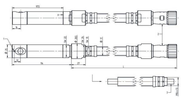
Dimensional drawing FFS08 with metal protection hose, FFS08 with extended housing comparable
