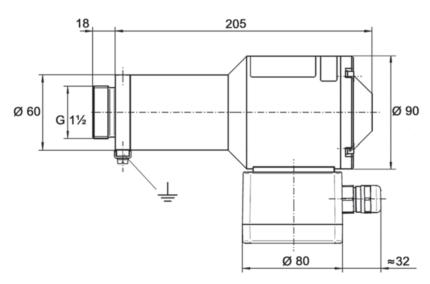
Dimensional drawing flame scanner F200K Ex with junction box
