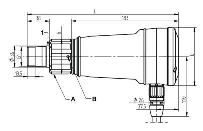
Dimensional drawing FV30-00 with flame scanner F300K
