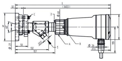
Dimensional drawing FV40-10 with flame scanner F300K
