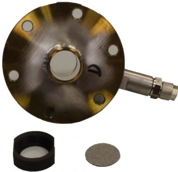
Fig. 7-7 Sensor holder with filter cap and filter
