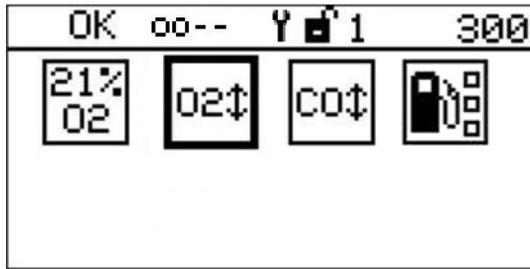
In Probe Calibration, select
