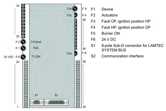
Fig. 6-3 Back view ETAMATIC V
