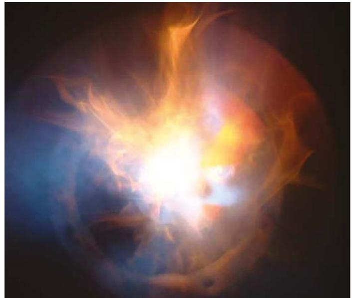
Efficient and safe combustion requires a precise mixture of fuel and air. CO<sub>e</sub> Control enables the burner to operate a fuel/air mixture on the edge of stoichiometric combustion in which exactly the right amount of oxygen molecules reacts with fuel molecules to complete the combustion reaction
