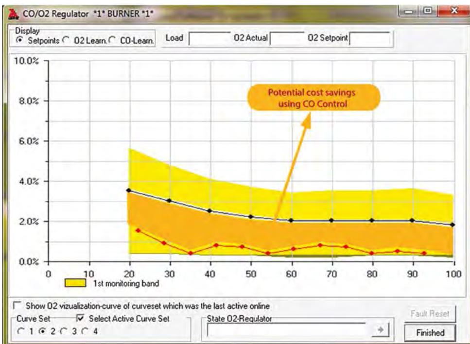
CO & O<sub>2</sub> curves with cost saving area highlighted between the two
